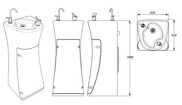
INLET: 860mm ABOVE BASE 100mm LEFT OF CENTRE LINE (from back) OUTLET: 860mm ABOVE BASE 30mm LEFT OF CENTRE LINE (from back)
